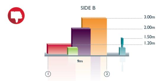
**Side B:** Between (1) and (2) there is no line of sight (opening), therefore the stand elements lower than 1,20 height (green and red elements) are considered as obstructive and will count in the calculation of the transparency.
