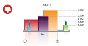
Side B: Between () and () there is no line of sight (opening), therefore the stand element lower than 1.40m height ( blue on the left side) is considered as obstructive and will count in the calculation of the transparency.
