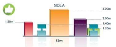
Side A: because there are lines of sight (opening) between the elements and we can see through the stand from aisle to aisle, the items less than 1.40m in height (blue and green on the above drawing) are not considered as obstructive and will not count in the calculation of the transparency.
