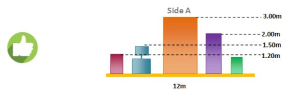
**Side A:** because there are lines of sight (opening) between the elements and we can see through the stand from aisle to aisle, the items less than 1.20m height (green and red on the above drawing) are not considered as obstructive and will not count in the calculation of the transparency.
