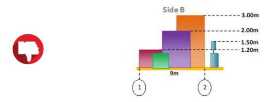
**Side B:** Between  $\binom{1}{2}$  and  $\binom{2}{2}$  there is no line of sight (opening), therefore the stand elements lower than 1.20m height are considered as obstructive and will count in the calculation of the transparency.
