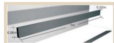
▶ R2. Ceiling aluminum beam to hold extra spotlight
