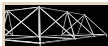
▶ Aluminum tube construction of 1.00x1.00m
