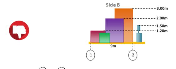
**Side B:** Between  $\begin{pmatrix} 1 \\ - \end{pmatrix}$  and  $\begin{pmatrix} 2 \\ - \end{pmatrix}$  there is no line of sight (opening) between the orange and violent structures. The total of both structure should not exceed 1/3 of the total length. The stand elements lower than 1.20m height are not considered as obstructive and will not count in the calculation of the transparency.
